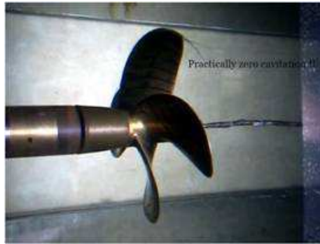
Fig. 3. Simulated nominal wake testing, in 850x850 mm section of the cavitation tunnel at 25 rps rotative speed (it can be remarked lack of cavitation).
