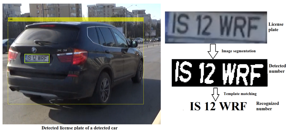
Fig. 2. Example of vehicle, license plate and number detection and recognition
